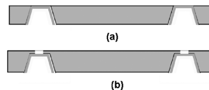
Fig. 9. (a) Showing via exposure directly by grinding and polishing. (b) Via exposure by combination of BG, polishing, and dry etching.
