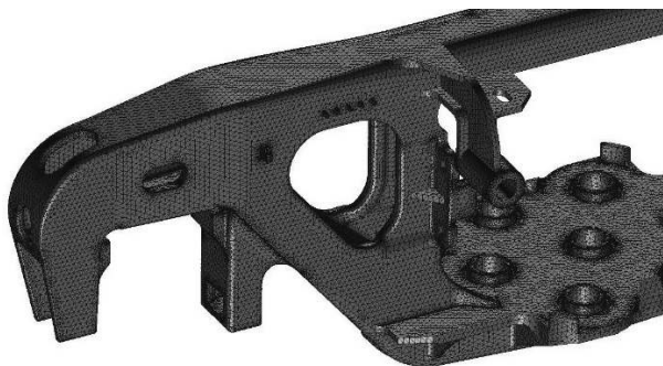
Fig. 6. Detail of finite element model of the bogie side frame with support surfaces
