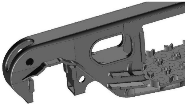
Fig. 1. Geometric model of ZK-1 bogie side frame
