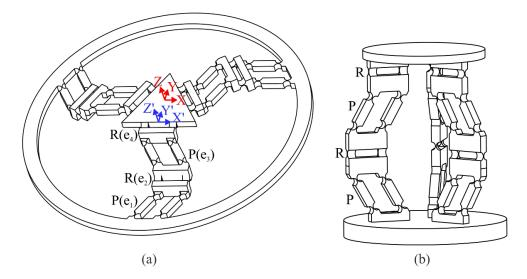
**Figure 8.** Prototypes of 3PRPR-CPMs with (**a**) *X*-*Y*-*Z* motions modeled based on the design presented in [24] and (**b**)  $\theta_X$ - $\theta_Y$ -*Z* motions modeled based on the design presented in [17], respectively.
