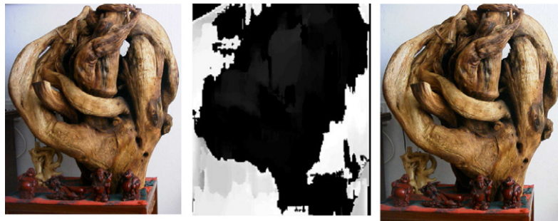
Figure 8. Stereo images (left and right images) and corresponding depth map (centre image). Although the resulting depth map does not show the exact metrics of the stereo pair, it is sufficient for the purpose of visualization.
