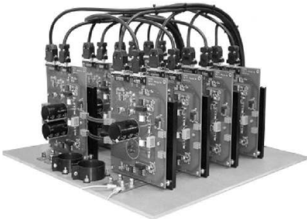
a) Photograph of the FCMI experimental setup
