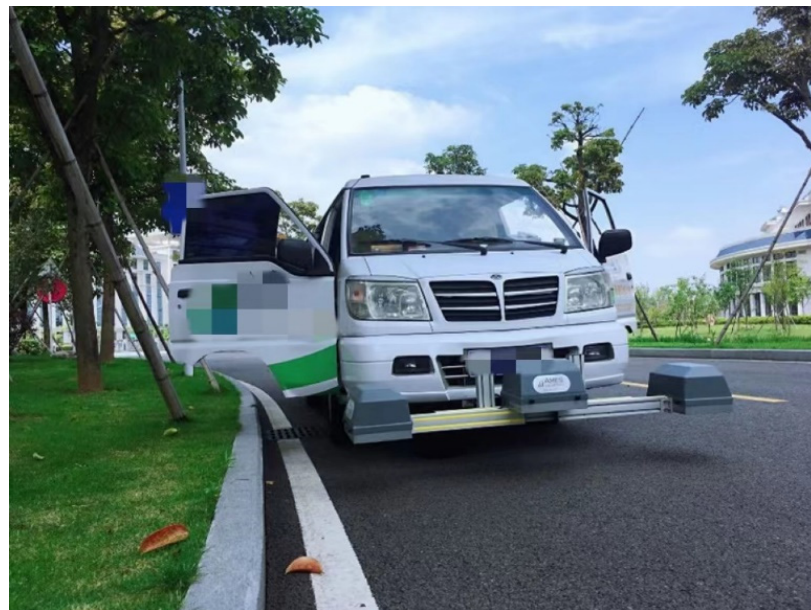
Figure 20. Road multi-function detection vehicle.
