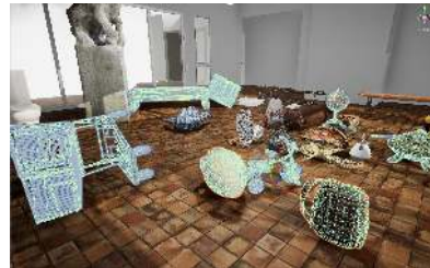
Figure 2: Green outlines around objects indicate auto-computed convex colliders for fast but accurate rigid-body physics.
