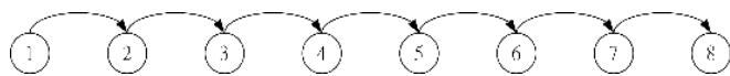
Figure 1. UDP traffic flow with node 1 as the source and node 8 as the destination in an 8-node multi-hop traffic flow
