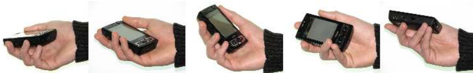
Figure 1: Tilting along the x axis: down , neutral , up and along the y axis: left , right .
