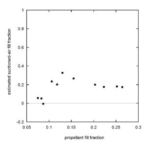
Fig. 22 Estimated volume fraction of air
