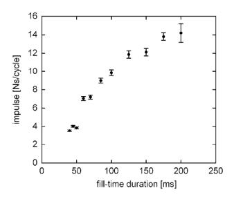
Fig. 18 Impulse versus fueling duration
