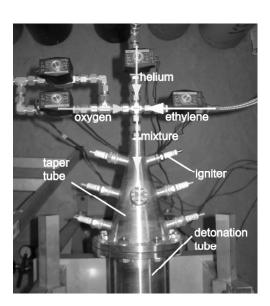
Fig. 3 Tapered tube and solenoid valves
