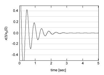
Fig. 11 Damping oscillation (c=250 Ns/m)
