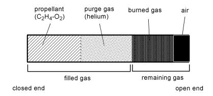
Fig. 21 Initial gas condition used in Endo's partial-fill model.
