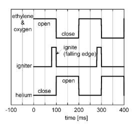
Fig. 4 Sequence A (mixture: helium = 1:1)
