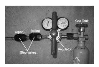
Fig. 14 Stop valves (connected)
