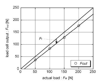
Fig. 7 Measurement of static friction
