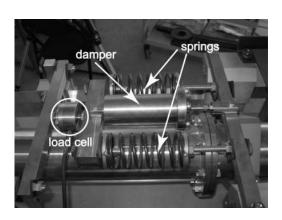
Fig. 8 Damping system
