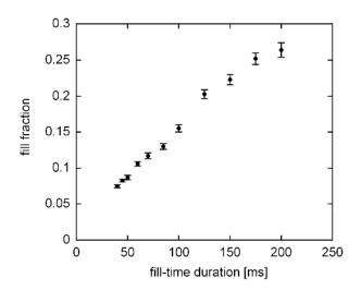
Fig. 16 Fill fraction of mixture versus fueling duration
