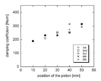
Fig. 13 Damping coefficient versus position of piston
