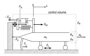
Fig. 6 Model for thrust measurement
