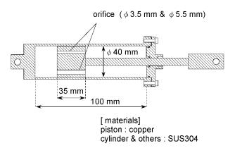
Fig. 12 Cross-section diagram of damper
