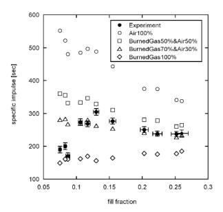
Fig. 20 Comparison of specific impulses between experimental results and Endo's partial-fill model calculation. The open symbols show model calculation results. "Air100%" or "BurnedGas100%" means that the remaining gas is air only or burned gas only, respectively. "BurnedGas50%&Air50%" or "BurnedGas70%&Air30%" means that a half or 70% of the remaining gas is burned gas and the other remaining gas is air, respectively.
