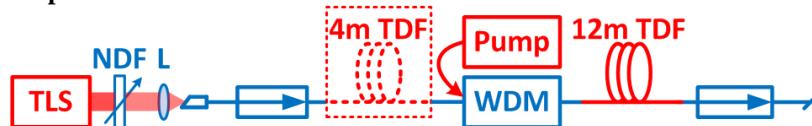
Fig.1 Schematic of the experimental setup. TLS: tunable laser source. NDF: neutral density filter. L: lens. WDM: wavelength division multiplexer. Improve display of pump, TDF, output
