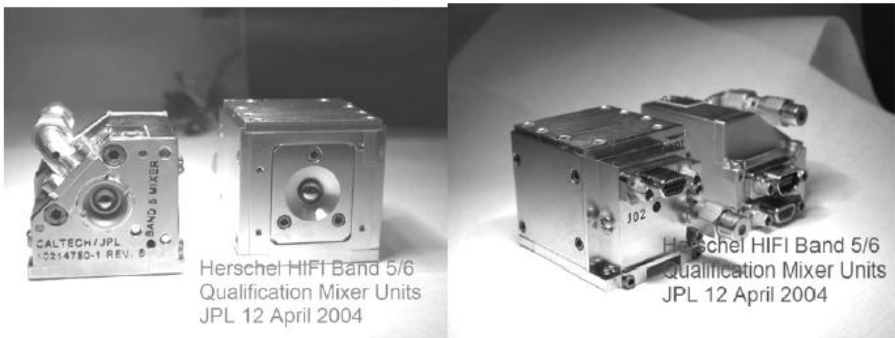
Figure 5: Qualification model band 5 and band 6 mixers
