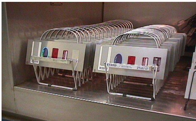
Figure 12. Adhesive Seals Inside Environmental Chamber
