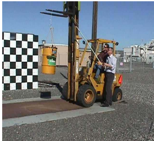
Figure 23. 113.56 L (30-Gal) Drum ready for Mechanical Shock Test
