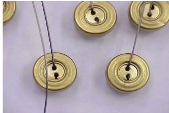
Figure 18. Elongation of E-Cup Wire Holes
