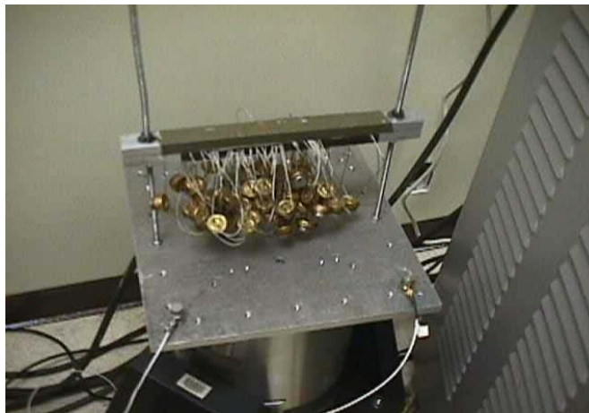
Figure 20. E-Cup Vibration Testing
