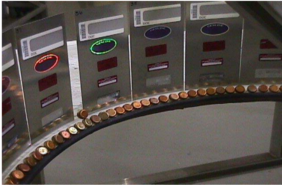
Figure 8. Adhesive Seals and E-Cups Around the South Exposure Station
