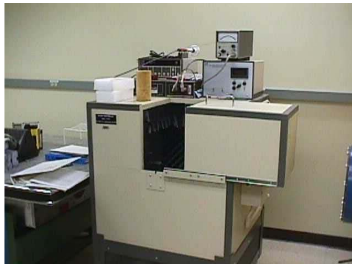
Figure 26. Microwave Test Chamber
