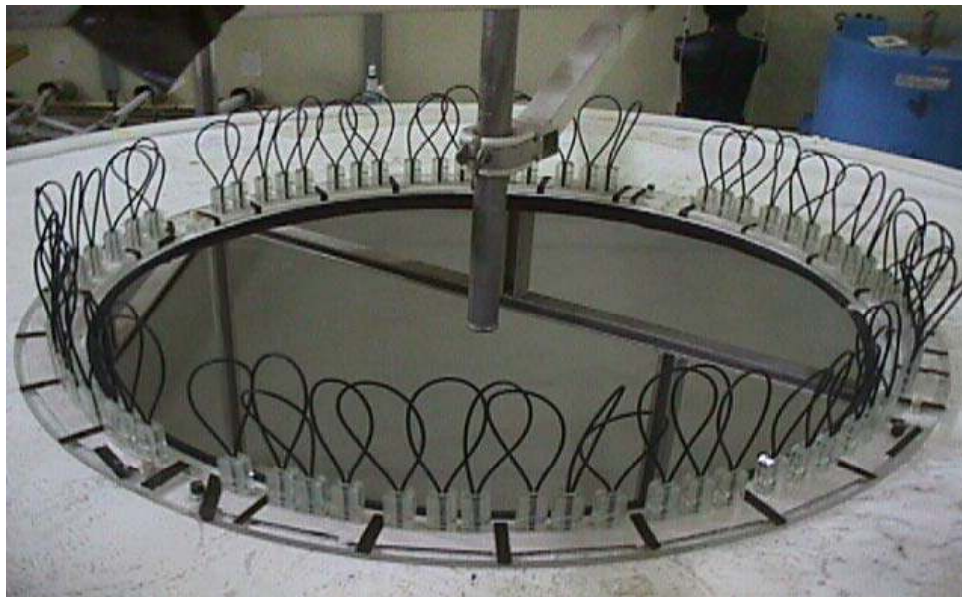
Figure 9. Cobra Seals Around the South Exposure Station
