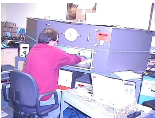
Figure 27. E-Tag Testing in RF Chamber
