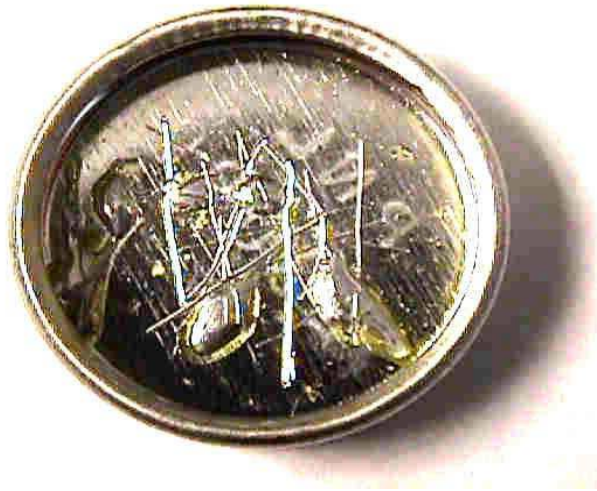
Figure 6. Bottom of a Prepared E-Type Cup Metal Seal
