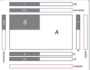
**Figure 3 Structure of TIGER models.** TIGER models are represented as Matlab structures. Boxes indicate size and orientation of the fields. Black text denotes TIGER field names. Gray areas contain data from the COBRA model, with white text indicating the relevant COBRA field names. Border color indicates data type: black → double-precision matrix, blue → cell array of strings, red → character array.
