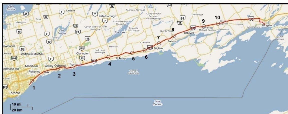
Figure 11. Road test trajectory from Toronto to Kingston. Circles indicate the locations of GPS outages.
