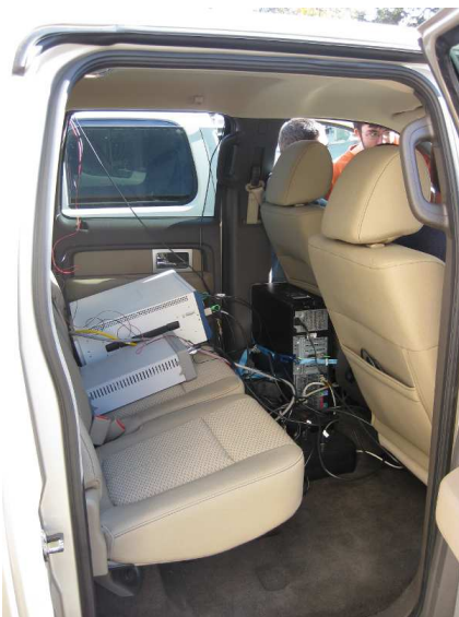
Fig. 5. The National Instruments RFSAs, RAID, reference clock, and computer placed in the back of the wardriving vehicle.
