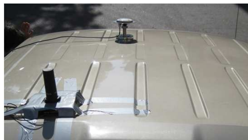
Fig. 6. Wardriving antennas placed on the roof of the vehicle.
