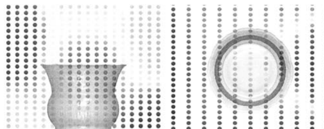
Figure 5. The variations in timbre around the object are mapped to grayscale (black is brightest, white is dullest) to visualize the spatial variations of sounds. Both images show the TimbreField produced by hitting the vase at the bottom right. The picture to the left depicts the brightness of the sound on a plane through the center of the vase. The picture to the right depicts the variations in a cross-sectional plane at the bottom.
