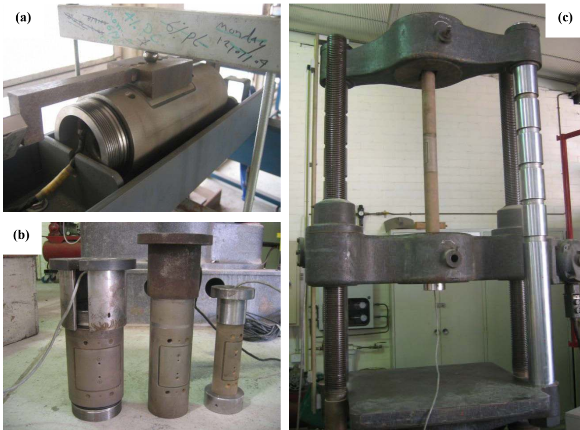
Figure A1. Calibration of the SSTs: (a) application of shearing and compression forces on the loading platen; (b) 135 mm, 100 mm and 65 mm diameter SSTs with top caps; (c) calibration of axial load sensitivity (in tension) using a Baldwin loading machine
