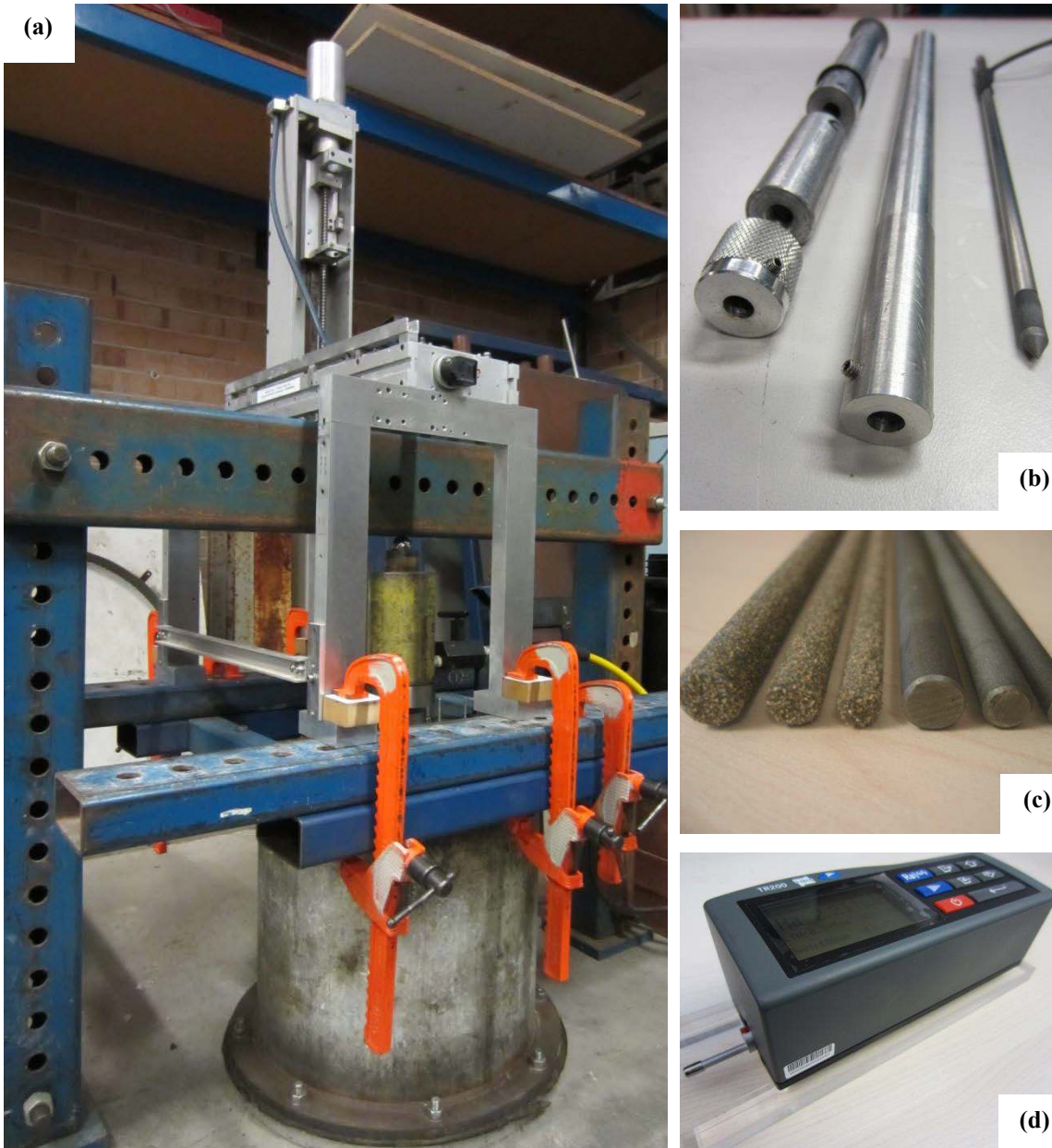
Figure 3.3. Setup of the experiment and the equipment used: (a) setup of experiment; (b) cone penetrometer; (c) model piles ; (d) roughness-meter
