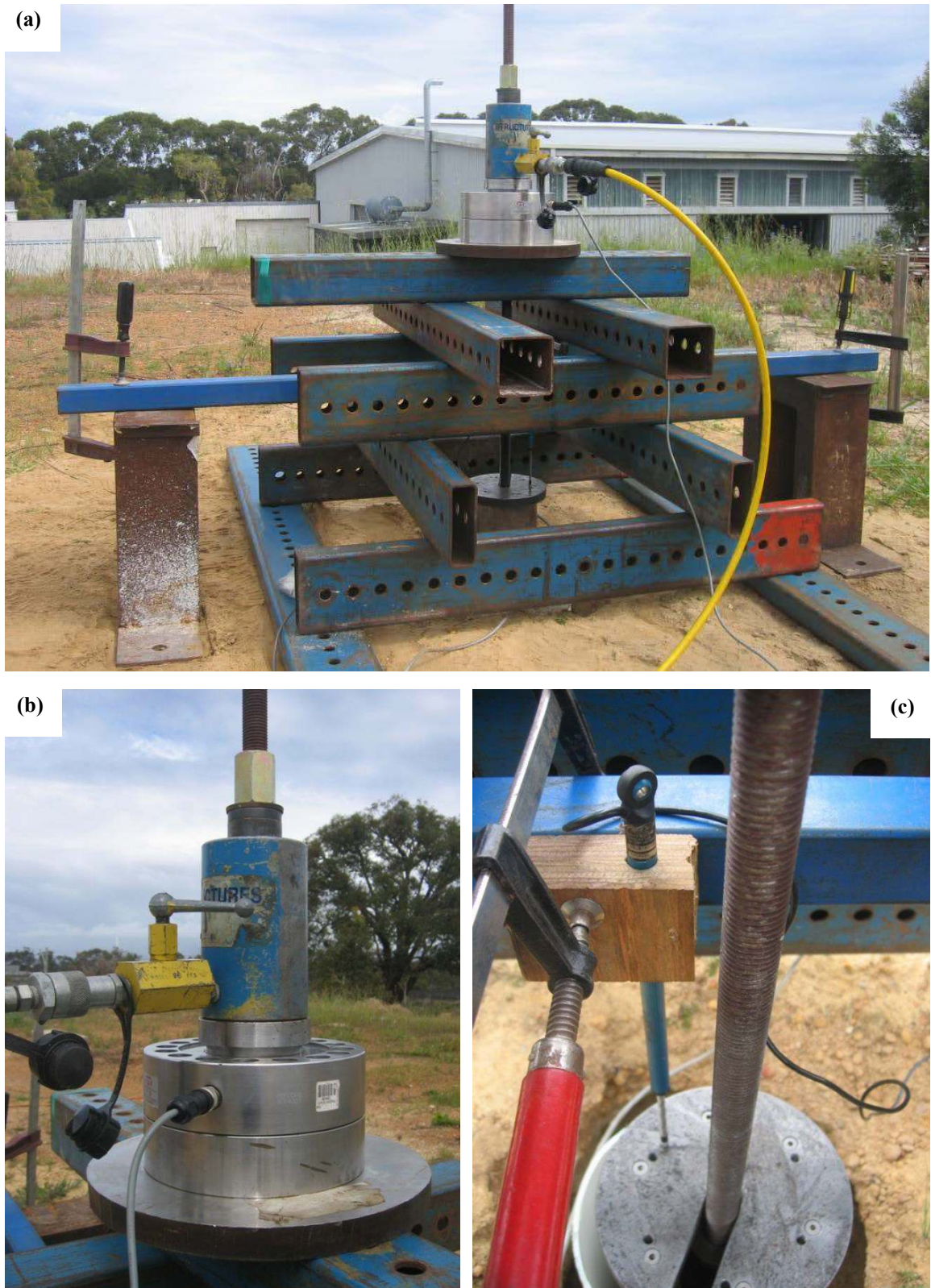
Figure 4.13. Tension load test: (a) overall test setup; (b) piston of the jack cylinder protruded during testing; (c) measurement of pile head displacement using LVDT
