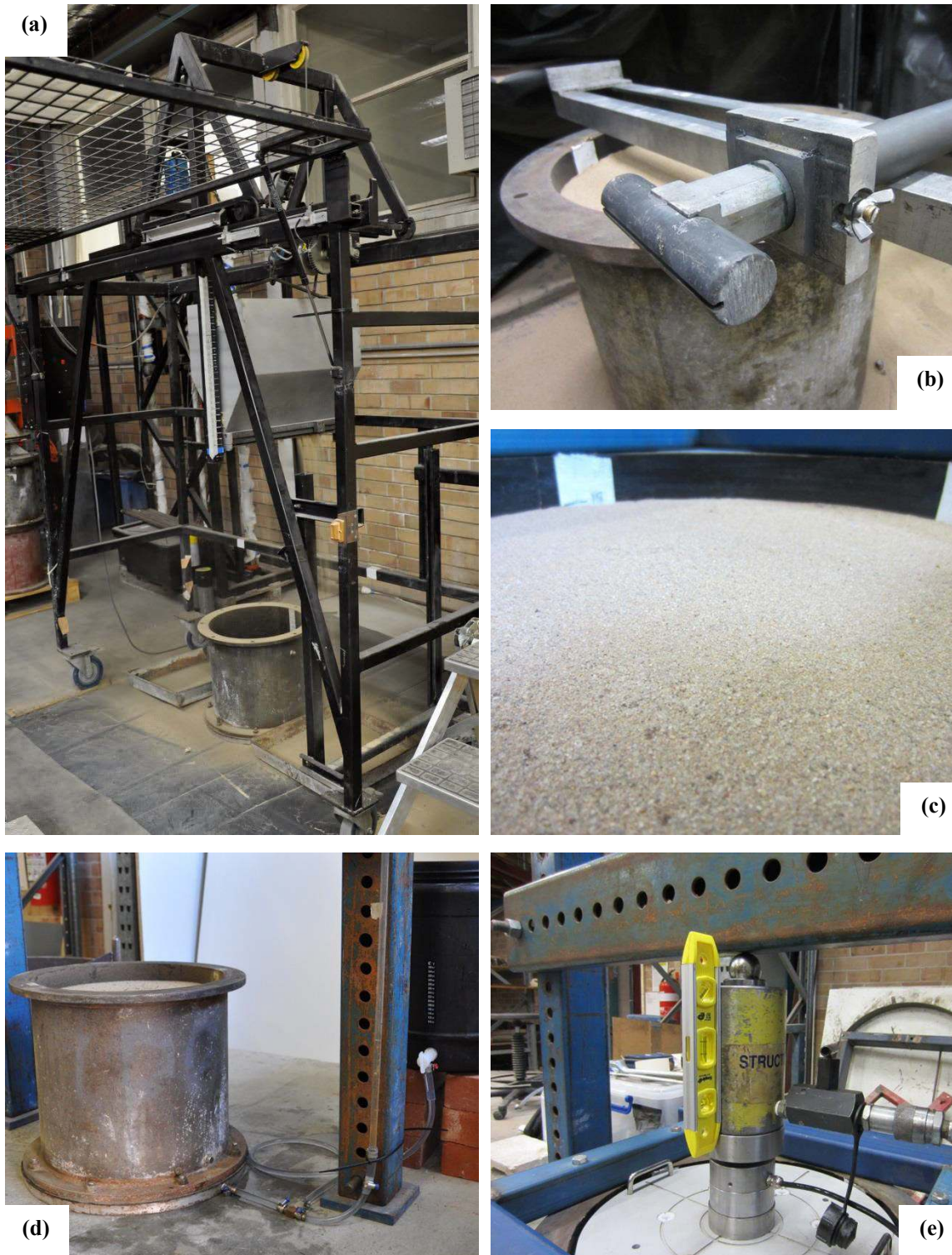
Figure 3.4. Stages of sample preparation: (a) sand deposition using automatic sand rainer; (b) vacuum device; (c) a levelled surface; (d) saturation; (e) pressurisation
