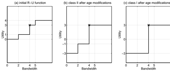
Fig. 3. Age modification for class I and II, with t_i^{age} = 5 , t_i^{max} = 10 , and actual bandwidth b_i = 4
