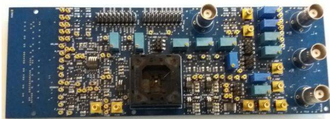
Fig. 12. Measurement printed circuit board which connects the sensor interface chip to the sensor electrodes.
