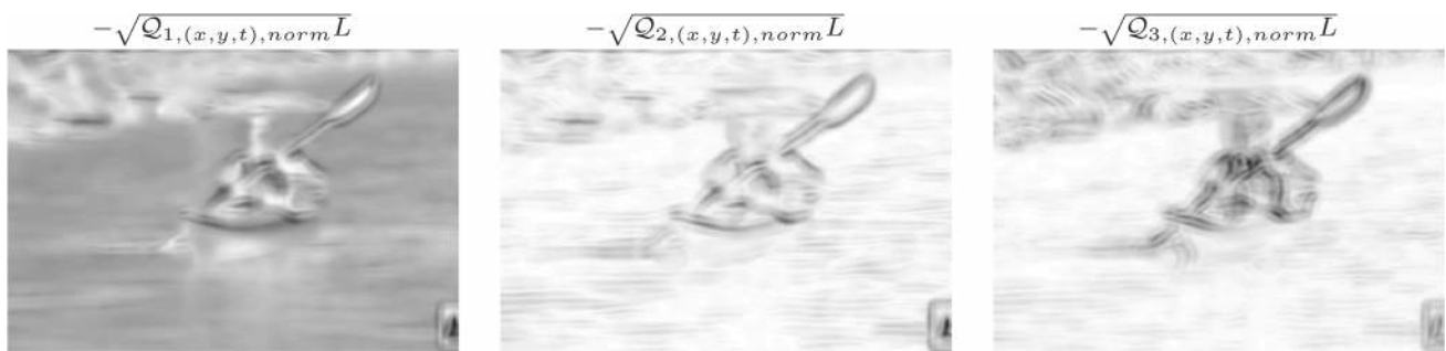
Fig. 8 Illustration of the influence of temporal illumination or exposure compensation mechanisms on spatio-temporal receptive field responses, computed from the video sequence Kayaking_g01_c01.avi (cropped) in the UCF-101 dataset. Each figure shows a snapshot at frame 8 for the quasi quadrature entity shown above the figure with additional monotone stretching of the magnitude values to simplify visual interpretation. Note how the time-varying illumination or exposure
