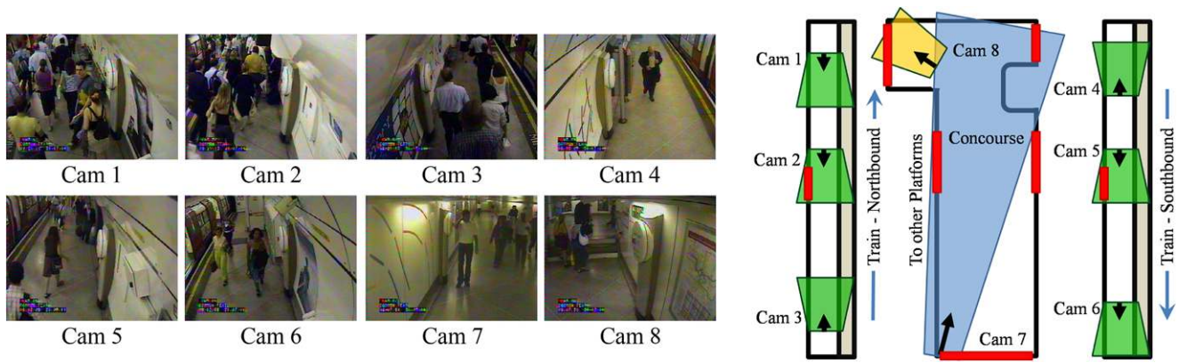
Fig. 5 (Color online) The station layout and camera topology of Station A dataset. Entry and exit points are highlighted in red bars
