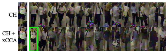
Fig. 20 Comparing person re-identification result obtained using CH+xCCA and CH alone. Given the probe image at the leftmost column, CH+xCCA found the same person in another camera view at rank 1, whilst CH can only find the true match at rank 59. Ambiguities due to similar visual features presented by multiple objects are greatly reduced by introducing time delayed activity correlation as contextual information
