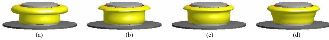
Figure 4. Isosurfaces of rv and \eta for fp_2 at s_x = 0.6 for full and m = 2 contribution as indicated; isolevel shown at rv = 300 , [\max] = [600] , rv(m = 2) = 5 , [\max] = [90] , \eta = \pm 300 , [\min, \max] = [-500, 500] and \eta(m = 2) = 180 & -60 , [\min, \max] = [-250, 350] . (a) rv ; (b) rv(m = 2) ; (c) \eta ; (d) \eta(m = 2) .
