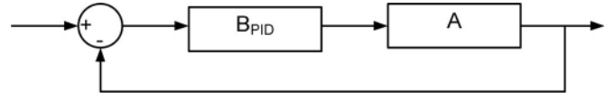
Fig. A4. Block diagram representation of the closed-loop system controlled by the desired compensator.
