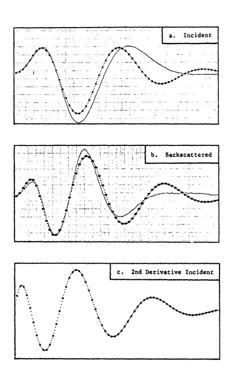
Figure 8. Comparison of an experimental result (solid line) with the theoretical prediction (broken line) for backscatter from a cylinder for ka = 0.32. The length of the abscissae is  $1 \mu$ sec for all graphs.
