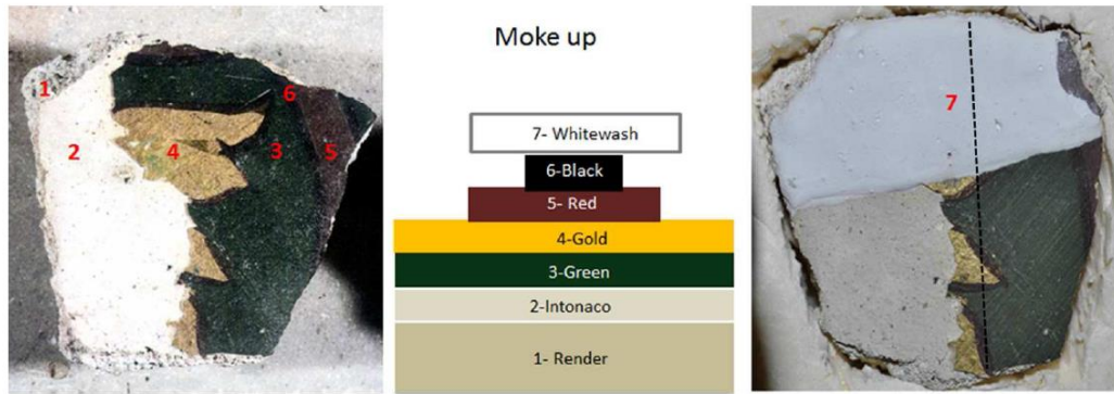
Figure 6: Sample without and with whitewash and its stratigraphy.
