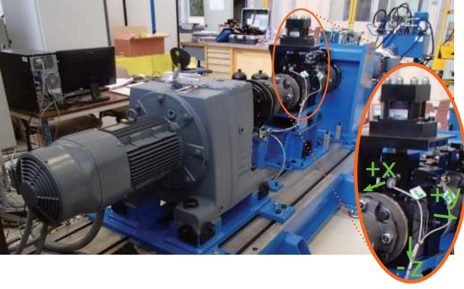
Fig. 6. A picture of the wind turbine test rig. The orange ellipsis circles the main bearing and its loading unit, while the green arrows represents the 3 wired accelerometers and their respective directions. (+ x ) and (+ y ) sensors are visible in the zoom, while ( -z ) sensor is hidden below the main bearing.
