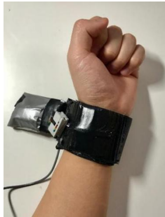
Fig 3-5. The BCG signal is measured by a developed capacitive wristband on the left wrist
