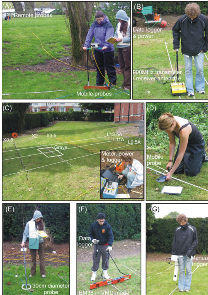
FIG. 3—Photographs of some near-surface geophysical equipment being trialed. (A) Bulk ground resistivity equipment; a Geoscan RM4™ lateral array. (B) High-frequency (900 MHz dominant frequency) GPR PulseEKKO™ 1000 equipment. (C) ERT electrode arrays ( \times 0.5 and \times 3.5 arrays laid out) using (inset) the CAMPUS TIGRE™ system. (D) SP survey using Pb-Cl probes and a standard voltmeter. (E) A Bartington MS.1™ magnetic susceptibility meter. (F) Bulk ground conductivity equipment: a Geonics EM38B™. (G) Magnetics equipment: a Geoscan FM18™ fluxgate gradiometer.
