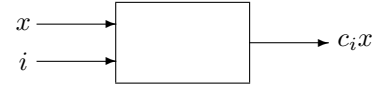
Fig. 1. The time-multiplexed multiple-constant multiplier block considered in this paper. The input x is multiplied by one out of N given fixed point constants c_1, \dots, c_N , based on the control input i .
