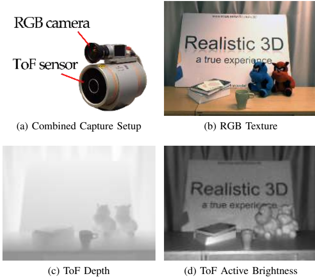
Fig. 1. Combined ToF+video capture setup (a) and its outputs: RGB Texture (b), low resolution ToF depth (c) and active brightness (d).
