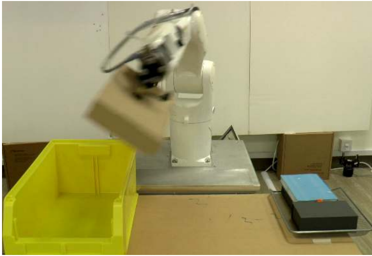
Figure 4.1.: Critically fast pick-and-place of a box with a suction cup. The full video of the experiment is available at https://youtu.be/b9H-zOYWLBY .
