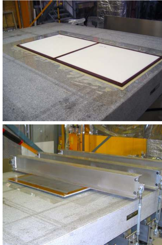
Figure 4: An inner box panel being laminated. The central FR5 bar provides a solid mounting point for the cathode.
