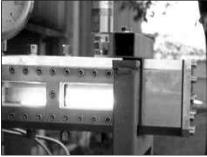
Figure 9 SPLab 2D slab hybrid burner rig during a combustion test
