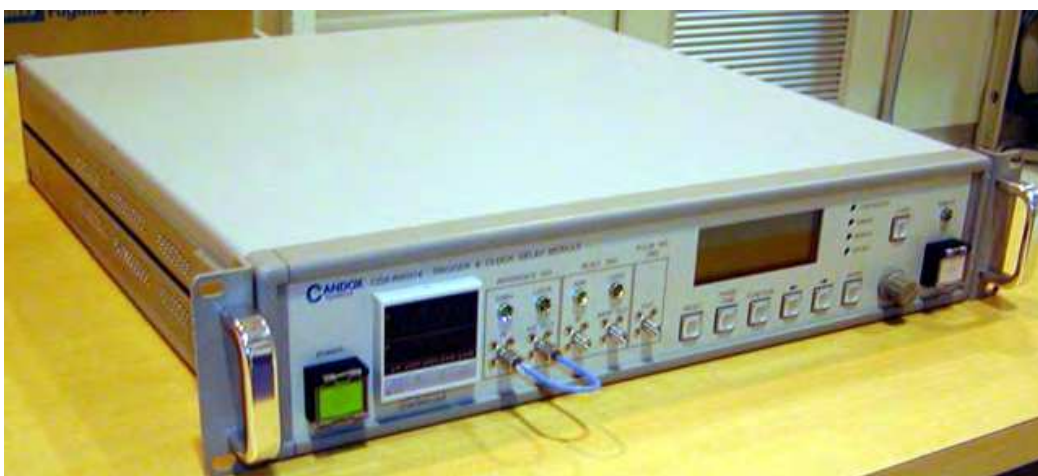
Fig. 6. High precision RF phase control circuit. The circuit provides a delayed RF signal from the output port with a precision of better than 3 ps (in rms) which is independent of the delay time.
