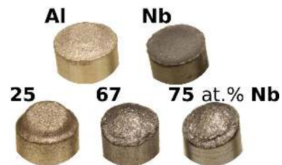
Figure 2. Eroded cathode surfaces of Al, Nb and the three compositions after approximately 10^4 arc pulses.
