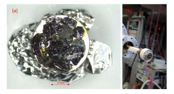
FIG. 10. (a)  $CsV_3Sb_5$  single crystals mounted on the HAL-9500 sample holder. (b) The sample holder with crystals attached to the cold finger of the continuous-flow He4 cryostat.
