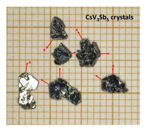
FIG. 1.  $CsV_3Sb_5$  single crystals used in muon-spin rotation/ relaxation ( $\mu$ SR) experiments. The crystallographic *c* axis stays perpendicularly to the flat surfaces of the crystals. The red arrows represent directions of the crystallographic *a* axis.
