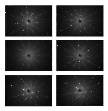
FIG. 7. The Laue x-ray images of the six  $CsV_3Sb_5$  single crystals presented in Fig. 1. The images demonstrate the single crystallinity of the material and correspondence of the main crystal axes to the sample shape.
