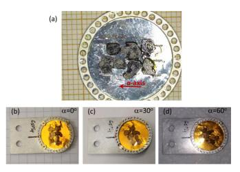
FIG. 9. (a) CsV<sub>3</sub>Sb<sub>5</sub> single crystals mounted on the holding ring of the GPS sample holder. [(b), (c), and (d)] The sample ring attached to the sample holder and turned at the angle  $\alpha = 0$  (a), 30 (b), and 60° (c), respectively.
