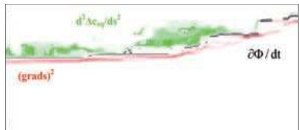
Fig. 20: Heterogeneous island. Regions of high values of (grad s)^2 (red), \frac{\partial^2 \Delta c_{eq}}{\partial s^2} (green), and change of porosity (black) in the modeling domain.
