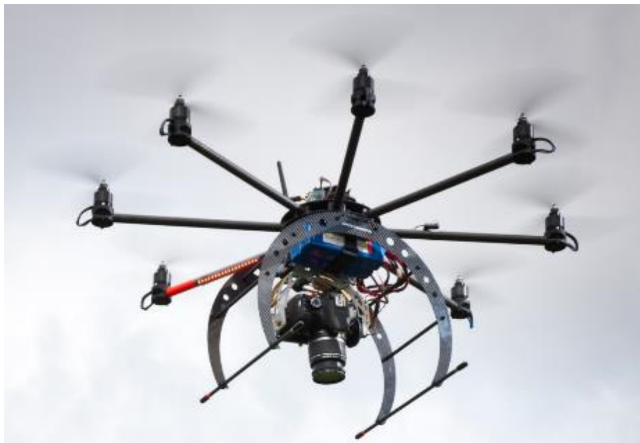
Figure 1. Oktokopter in flight, fitted with Canon 550D camera.
