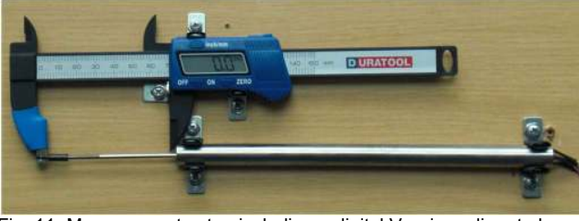
Fig. 11. Measurement setup including a digital Vernier caliper to know the actual position of the core inside the displacement sensor.
