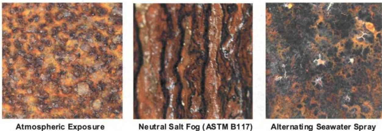
Figure 11: Examples of 1010 steel (UNS 10100) panels after prolonged exposure to atmospheric (top left), alternating seawater spray (right), and neutral salt fog (bottom left) environments.
