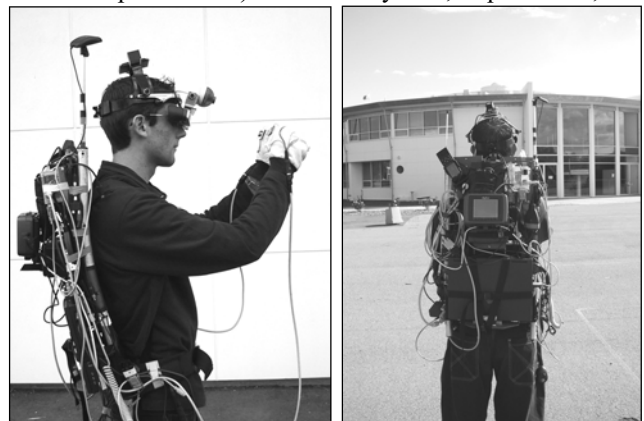
Figure 6 – (1) Tinmith wearable computer, with glove input devices (2) Rear shot located near example school building, facing west
