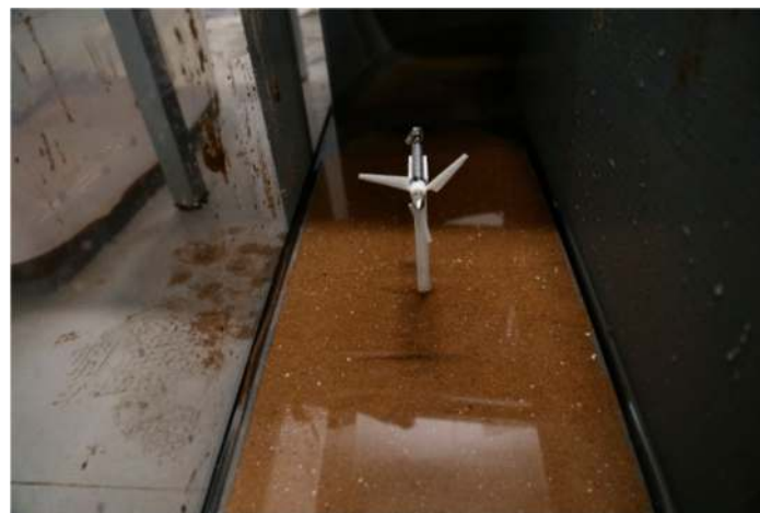
Figure 7. 3D printed turbine model and monopile structure for the scouring experiment.
