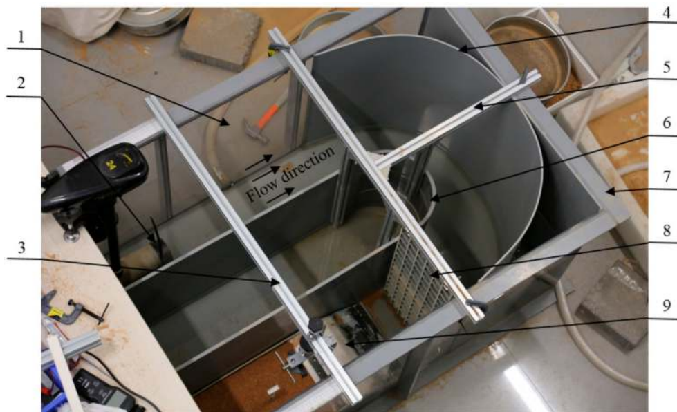
Figure 6. Recirculating flume in Marine Renewable Energy Laboratory, Tianjin University. (1: Plexiglass; 2: Propeller; 3: Laser range finder; 4: Guide bend; 5: Frame structure; 6: Separator; 7: Flume; 8: Perforated distribution plate; 9: Sand box).
