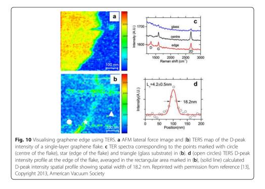
contaminated areas within a graphene flake with sub-diffraction-limited resolution, which otherwise cannot be resolved with confocal Raman spectroscopy.
