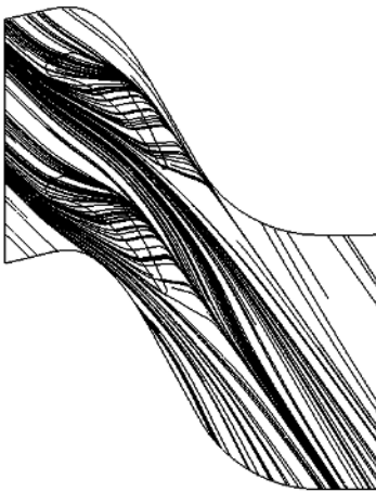
Figure 13. Streamlines over the blade tip for three different speeds.
