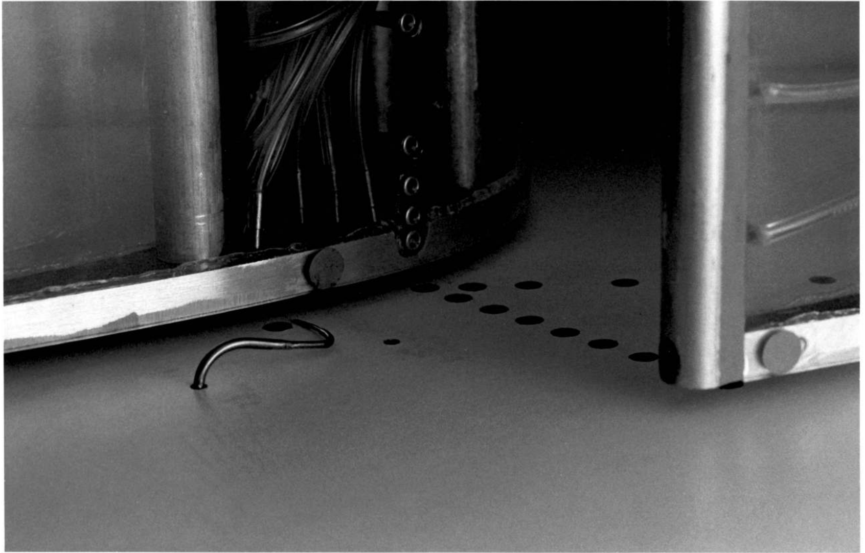
Fig. 19 Pitot Probe B at Tip Gap Exit.
