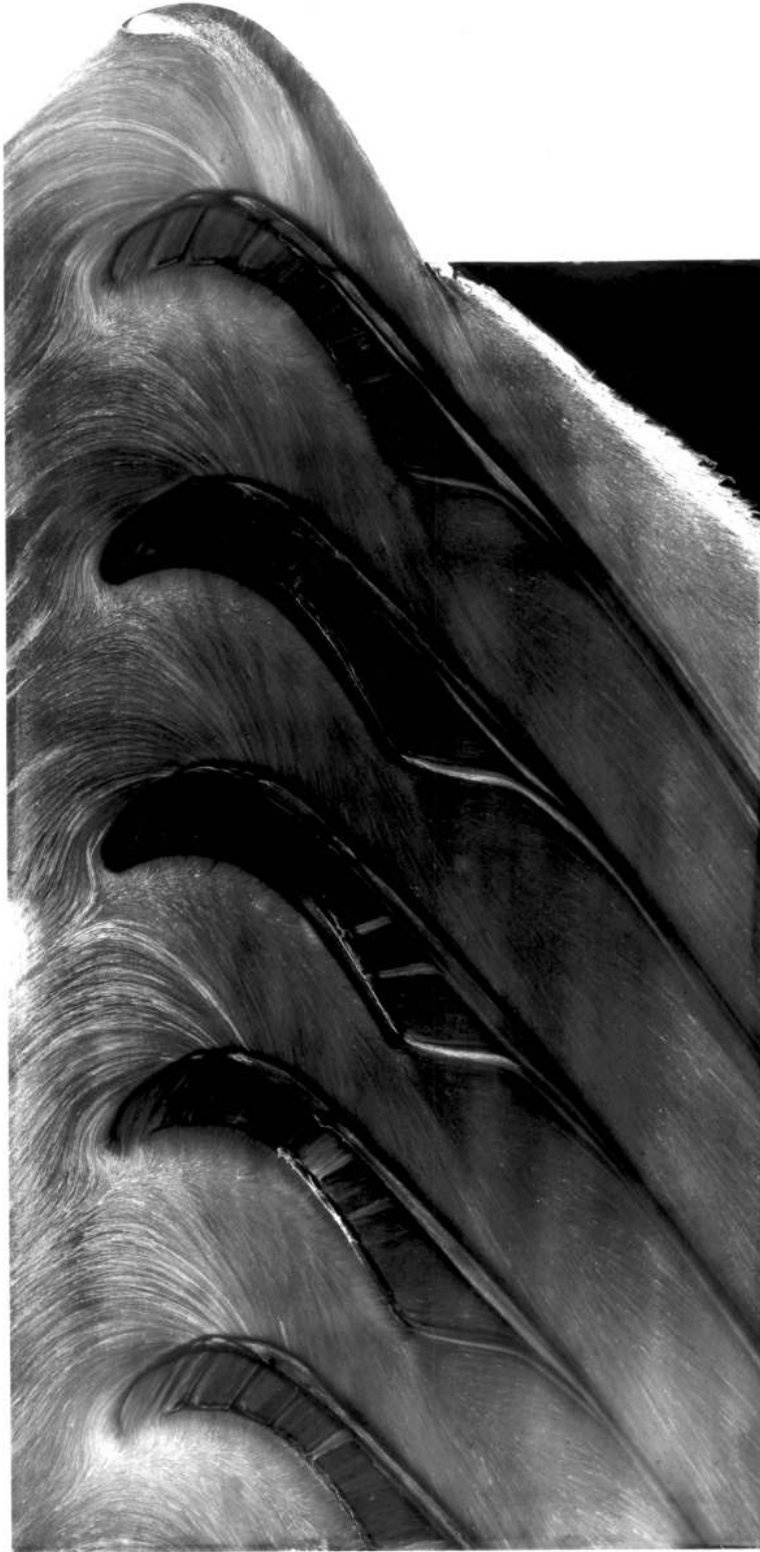
Fig. 20 Bottom Endwall Flow Visualization.
