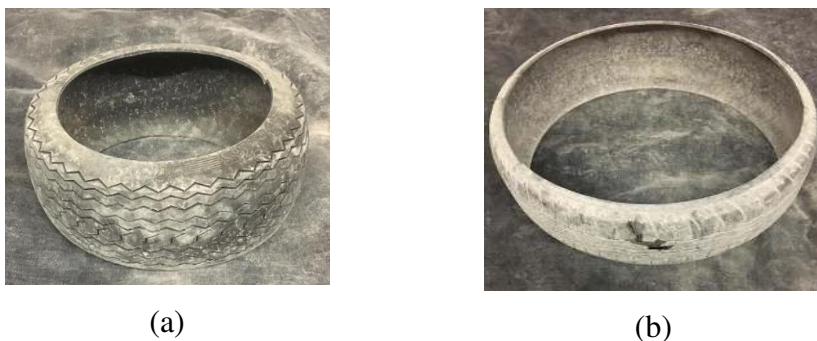
Figure 3. 17 Tire-derived geo-cylinders (TDGC) (a) small geo-cylinder (~16” diameter), or TDGC-S (b) large geo-cylinder (~24” diameter), or TDGC
