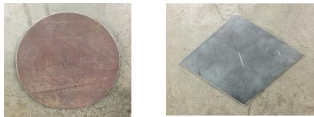
(a) (b) Figure C. 1 Loading plates utilized while testing for confinement (a) 11" diameter plate (b) 40 in 2 surface area plate
