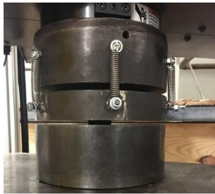
Figure 3. 21 Compression testing of the TDGC specimen
