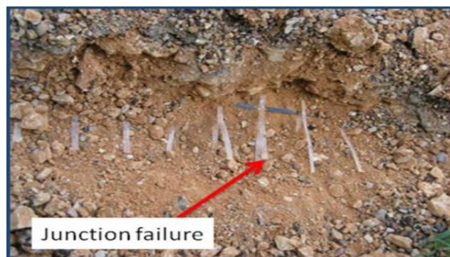
Figure 2. 11 Separation of longitudinal and transverse ribs at junctions of Geogrid B at location FM 1774 (Zornberg et al. 2015)
