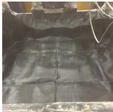
Figure 3. 11 Reinforcement woven geotextile utilized for base/sub base support
