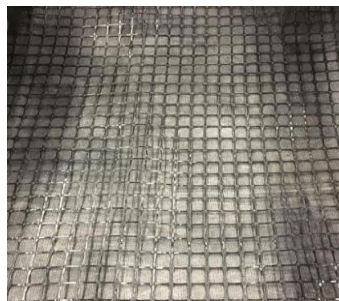
Figure 3. 13 Geogrid specimen utilized for base/sub base support
