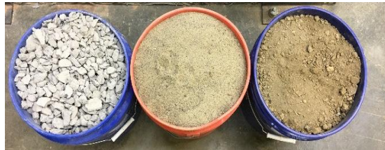
Figure C. 2 Infill Materials (AASHTO #57 Aggregate, sand, SM-soil) for filling TDGCs and geoweb for confinement tests
