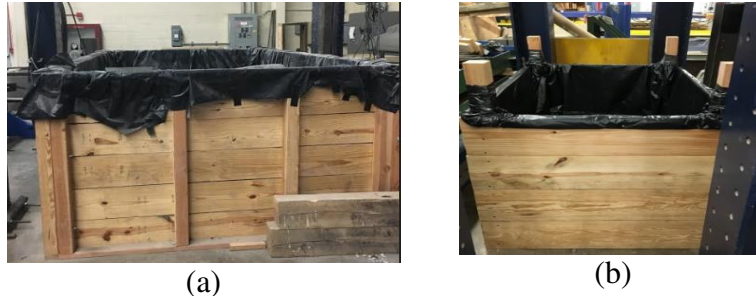
Figure 3. 27 Representative pavement (roadway) section set-up (a) large bin, 7' x 12' (b) small bin, 4' x 6'
