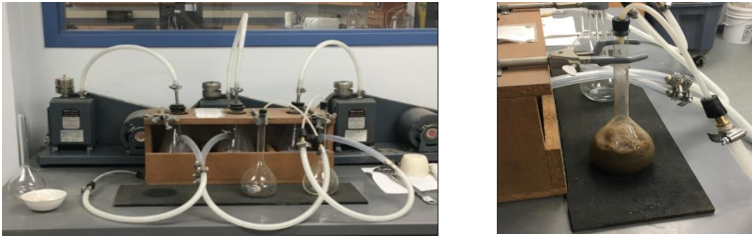
Figure 3.7 Specific gravity testing of the subgrade soil specimen (a) pycnometer used for soil testing (b) air being withdrawn from the soil specimen.
