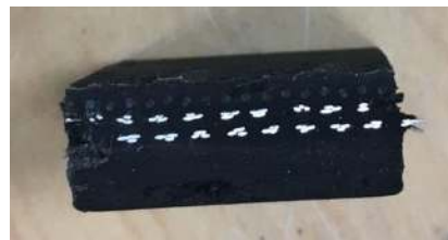
Figure 3. 20 TDGC specimen used for compression testing
