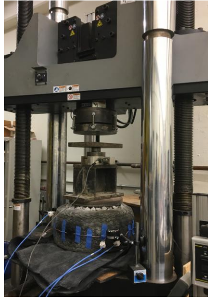
Figure C. 6 Confinement testing of instrumented TDGC-S
