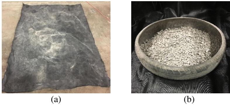
Figure 3. 10 Separation woven fabric (a) fabric used on top the subgrade for the large and small test bins (b) a TDGC placed on top of the separation woven geotextile fabric
