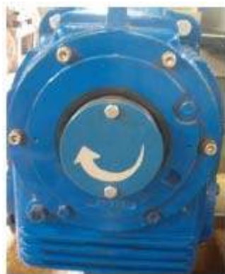
Figure 6-7 The arrow direction imprinted on the high-torque gear box indicating the shearing direction of the lower box.
