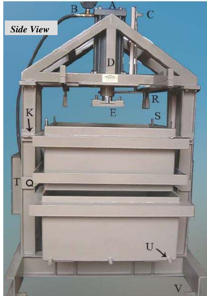
Figure 6-4 Front view of the DS box.
