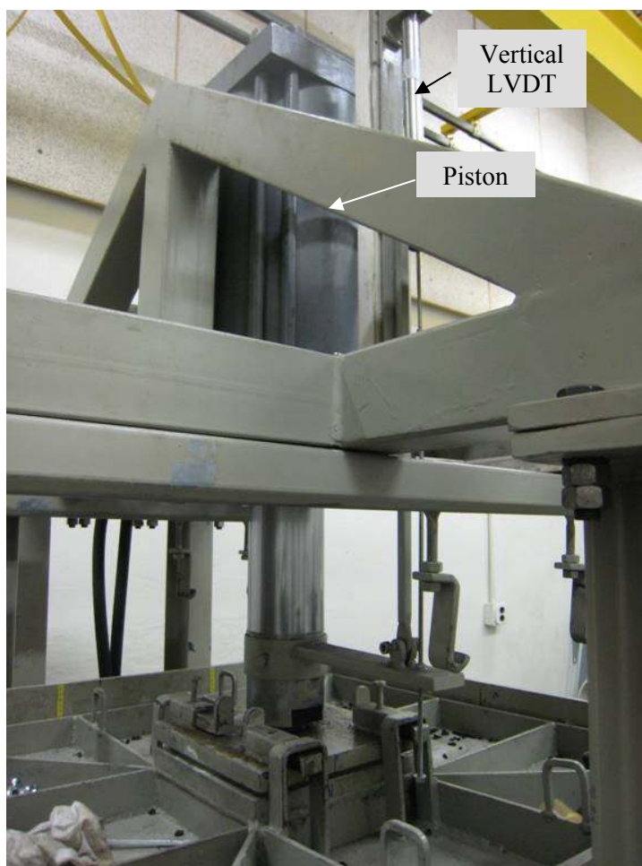
Figure 6-11 Vertical LVDT in position.
