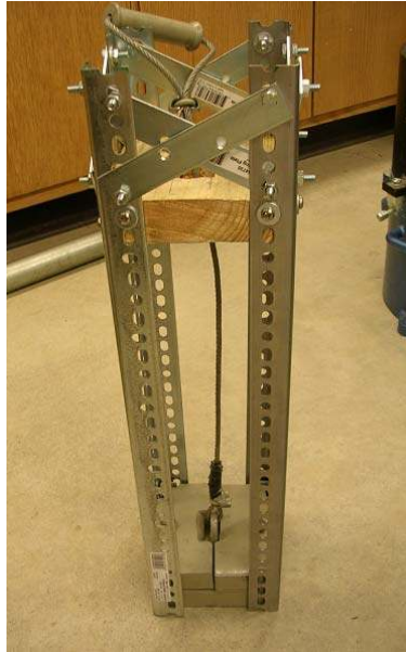
(a) Specially designed rammer
