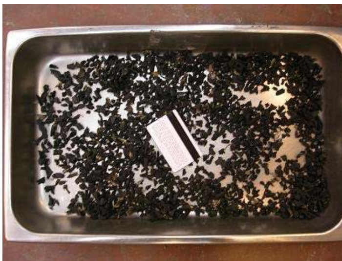
(a) Tire chips 9.5 mm in nominal size
