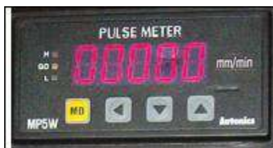
Figure 6-6 The lateral speed detector programmed to show the lateral speed of the lower box in mm/minute.
