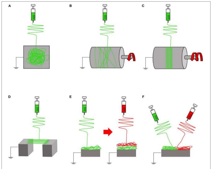
FIGURE 3 | Electrospinning setups to produce nanofibrous mats. (A) Flat plate collector (random nanofibers). (B) Rotating drum collector (rotational speed < 8 m/s = random nanofibers). (C) Rotating drum collector (rotational speed  $\ge 8$  m/s = aligned nanofibers). (D) Gap collector (aligned nanofibers). (E) Multilayer electrospinning configuration. (F) Co-electrospinning setup.
