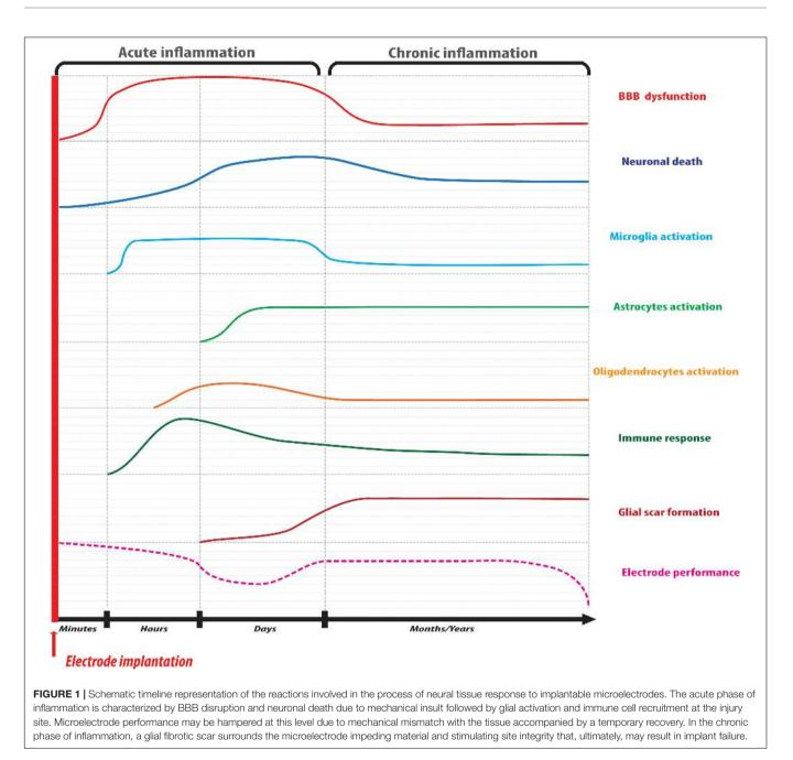
of proinflammatory cytokines and glial fibrillary proteins deposition by microglia and astrocytes, finally forming the glial scar (**Figure 1**). As a consequence of this neuronal death at the tissue-electrode interface, the distance between electrode and synapses grows in time, hampering electrical stimulation performance.
